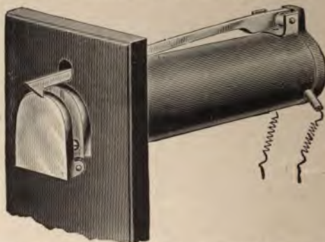
FIG. 116.—A typical Switchboard Line drop; the Tubular Drop of the Keystone Co. The iron tube contains an electro-magnet, to whose coil the current is admitted by the wires, as shown. The armature is hinged at the rear of the tube, and when it is attracted raises the longitudinal lever, thus releasing the shutter.
